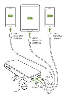
If you have USB-C devices, connect them to the powerstation, powerstation XL or powerstation XXL battery's USB-C connector for faster charging (up to 3 amps).
