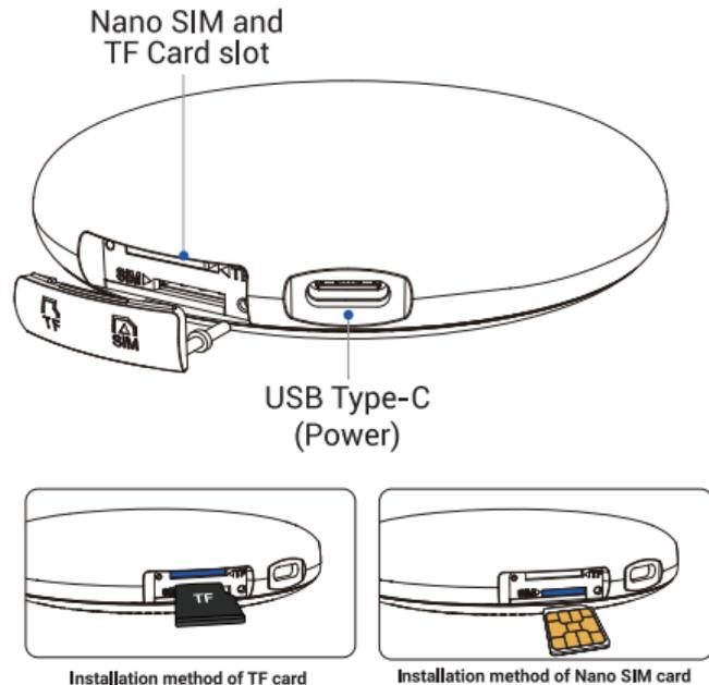
**Tips!** Power off before inserting or removing the nano SIM card. Nano SIM card and TF card are not included in the package. For how to insert the cards please refer to this diagram.
