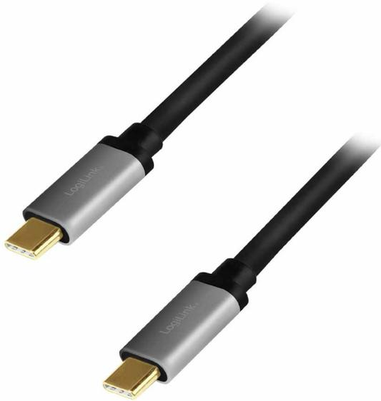
This USB-C cable built-in E-mark chip supports the devices intelligently to deliver the fastest charging up to 20 V/5 A (100 W) and provides the data transfer up to 480 Mbps.
