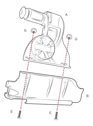
2 Use (D) Machine Screws and (F) Nuts to connect holder to any RAM® Mount
